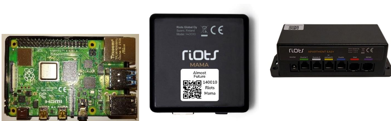
Figure 23: Raspberry Pi4, Riots mama device and apartment sensor
