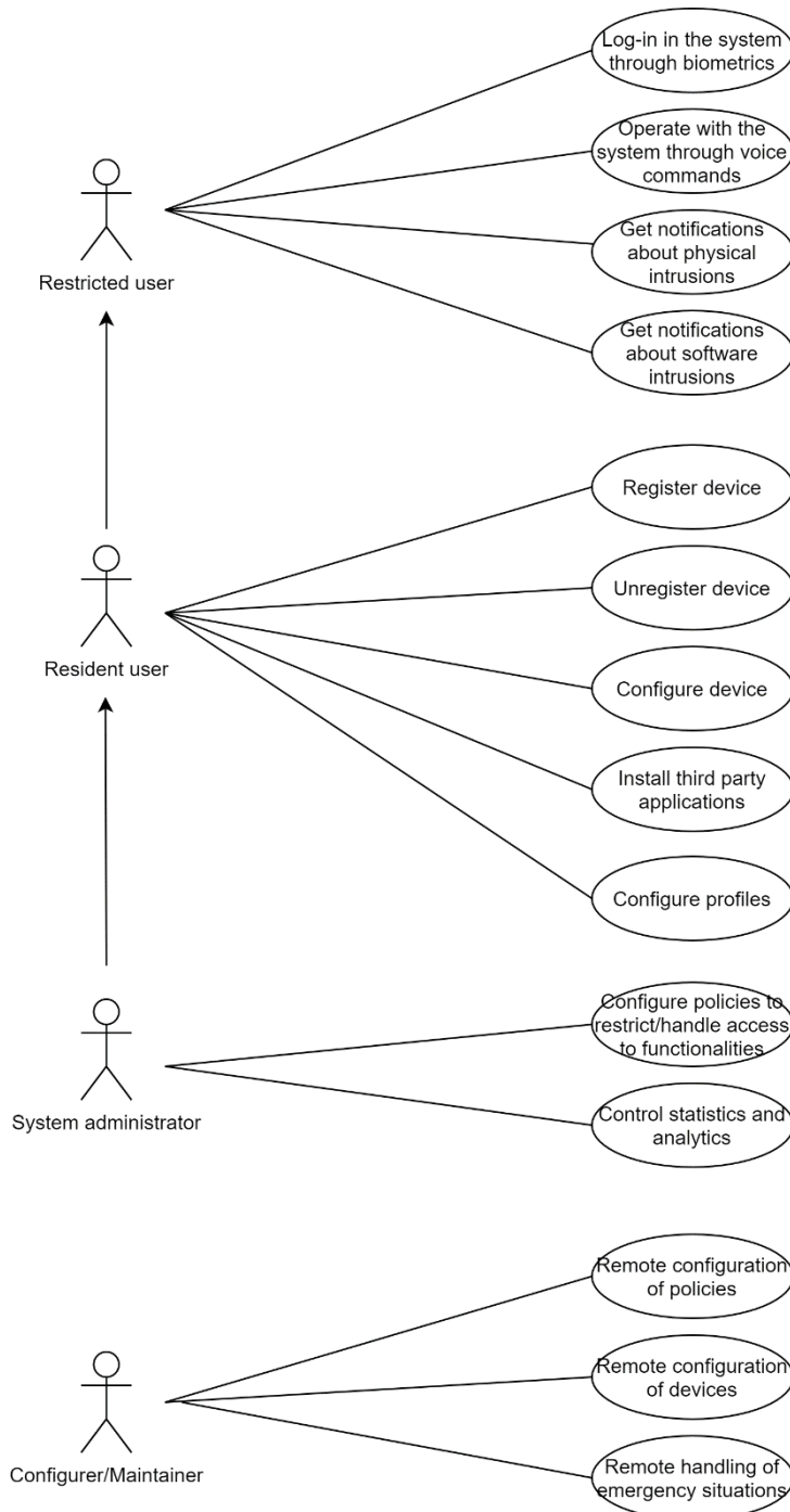
Figure 11. The full use case diagram of the SIFIS-Home system
